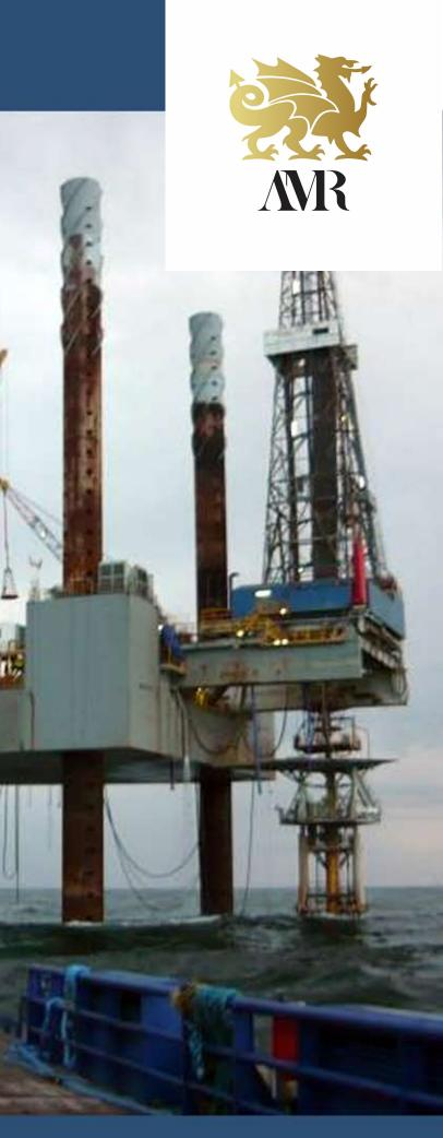
The GAEA 3 is a Bethelehem designed JU-200MC mat-supported cantilevered Jackup rated for operation in water depths of up to 200 ft and drilling depths of up to 25,000 ft. The GAEA 3 is ready for transport from the USA to its required location as and when it is needed. 99
